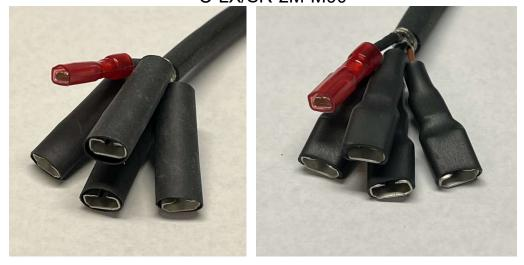
7) Slide lugs on the connector on the end that does not spin. Reference Figure 1.
