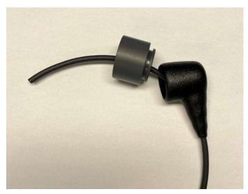
3) Slide a 3" piece of 3/4" heat shrink on the cable.
