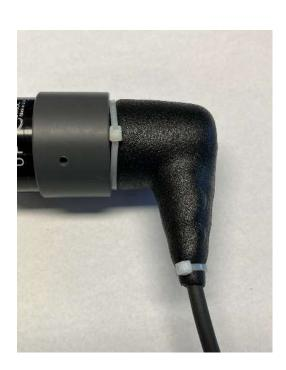
11) Attach (2) cable ties over the edge of the rubber boots.
