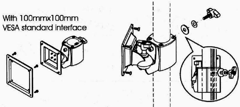
When the joint loosens ,tighten the parallel knob up with clockwise direction.
